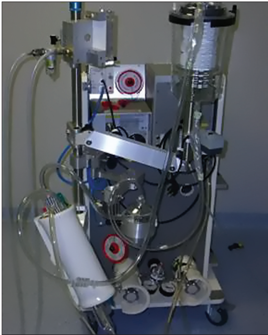
Figure 3. Heart-lung machine employed for percutaneous cardiopulmonary support
